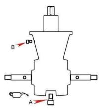
Check the oil in the leg annually. Change if necessary: oil drain plug under the anode (A). Oil level screw on the side of the leg (B). Copper washer should be changed. The anode should be checked frequently and changed if necessary (at least once a year). If you find water in the oil, it is necessary to change the propeller shaft oil seals. The anode must be checked frequently and changed if necessary (at least once a year).
