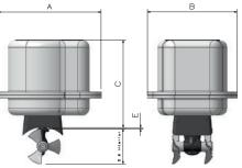
Certified ISO 8846, the CT35-IP is part of Max Power's Ignition Protected tunnel thruster range which allows the safe use of an electric tunnel thruster in petrol / gas engine vessels. IP thrusters are also ideal for installation in habitually wet or damp areas such as sail lockers or in the transom of deep «V» shaped motor yachts. The single propeller CT35-IP has a 125mm diameter tunnel and a thrust rating of 35 / 77 (kgf/lbs).
