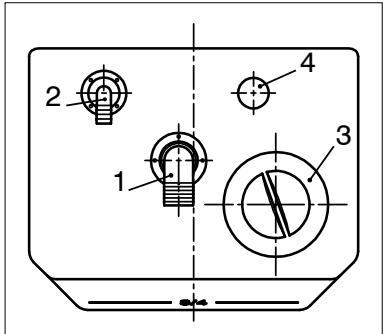
If necessary loosen the nut with the spanner supplied in order to turn the fittings to the required direction. Remember to tighten up the nut properly afterwards.
