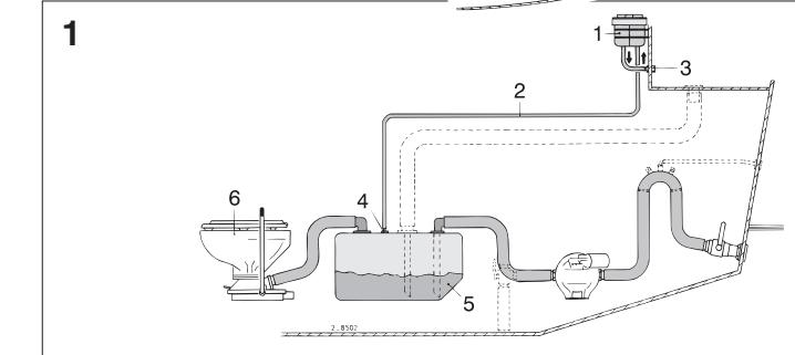
**Installatie beluchtingsleiding****Vent line installation****Installation Entlüftungsleitungen****Installation de la conduite de ventilation****Instalación del tubo de aireación****Installazione della condotta di aerazione**
