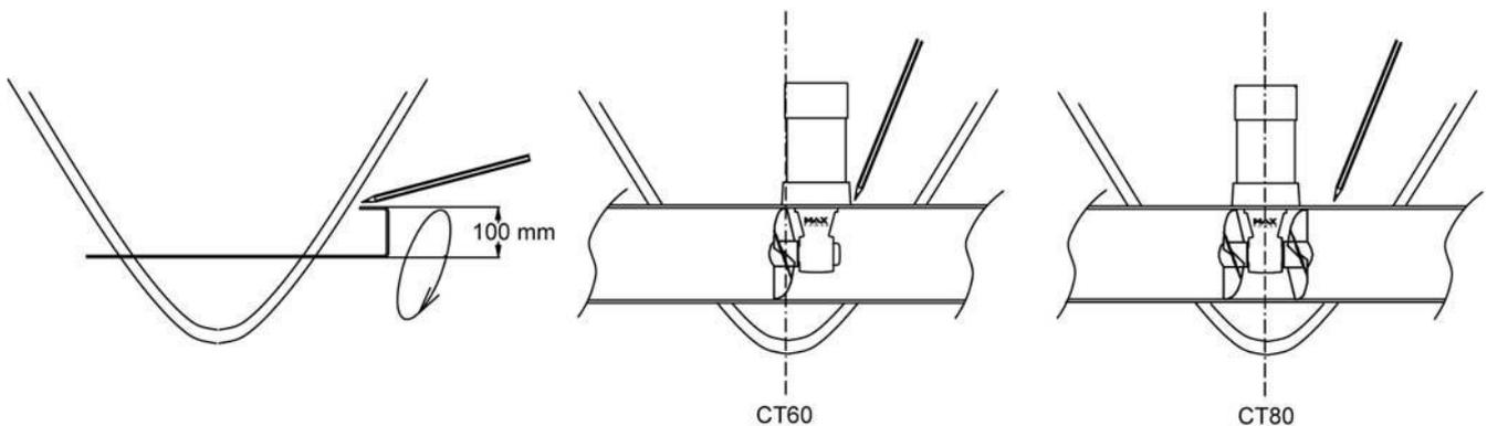
Replace the tunnel. To secure its position apply reinforced fiberglass filler to all areas, both inside and out, taking care to entirely fill the space between the hull and the tunnel. Laminate using a minimum of 8 layers of **ISOPHTALIC RESIN** alternated with mat and roving.
