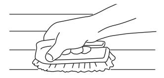
Use a brush to loosen debris inside of the old seam.
