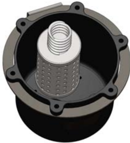
Figure 24. Oil filter spring
