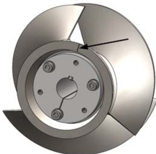
Figure 32. Position of the keyway
