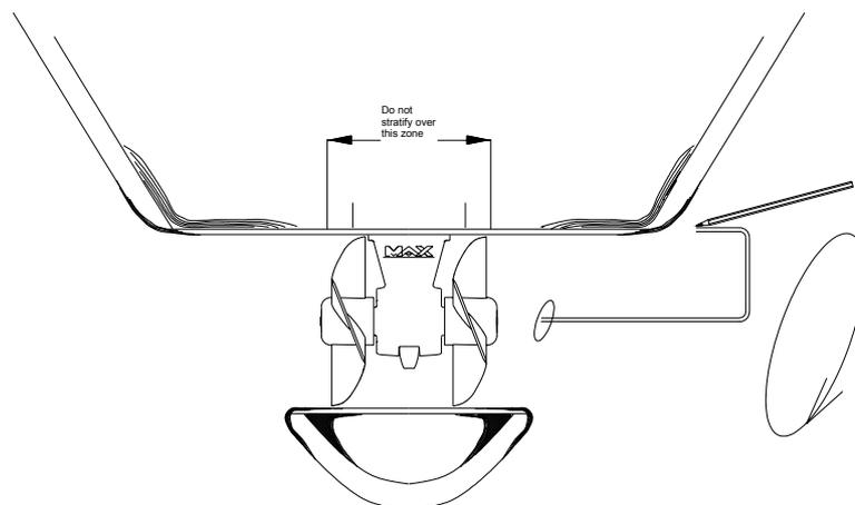
Fit the tunnel and mark the areas to be fibre-glassed. Sand these areas inside and out.
