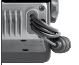
Wiring Located at Back of Radio
