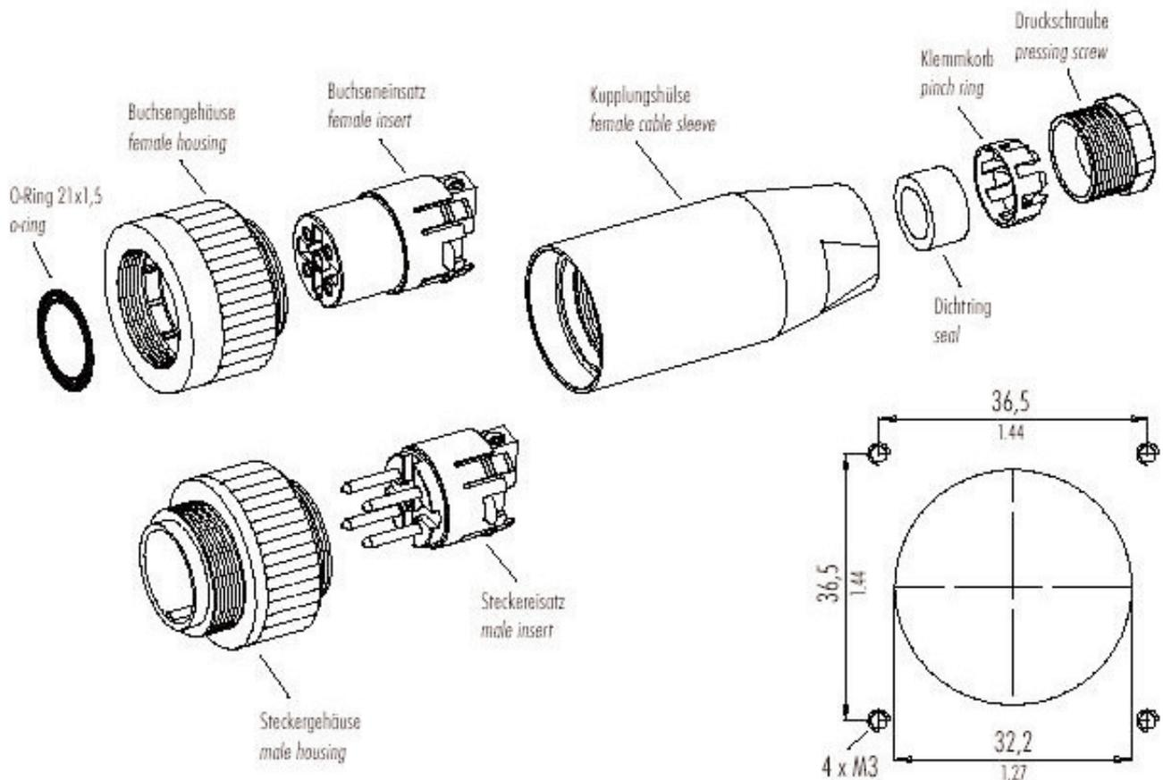
Cut-out dimensions for flange-socket or -plug
