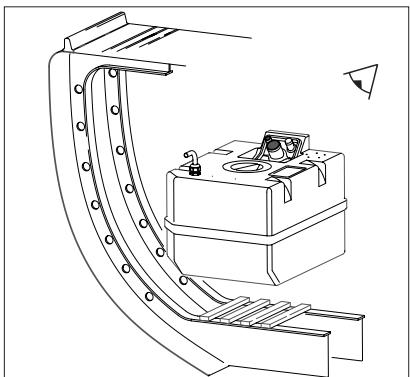
Ensure that there is a sufficiently solid foundation for placing and fixing the tank firmly.
