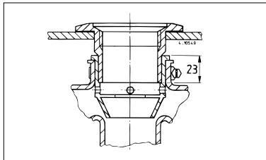
The top side of the Splash-stop is equipped with a connection for the breather line. This connection has a turning radius of about 200°.
