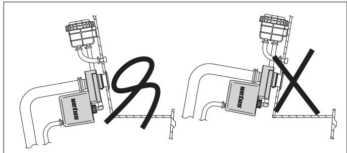
The bulkhead should be diagonal so that the Splash-Stop's filler cap is at a minimum angle of 10°.
