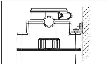
**Fit a filler hose** between the Splash-Stop and the tank. Use fireproof hose with a 38 mm or 51 mm inner diameter respectively. Place it such that no mechanical stress is placed on either the tank or the Splash-Stop.
