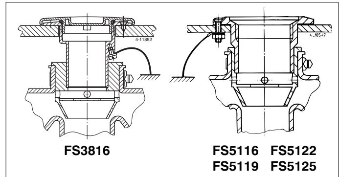
The deck fitting and the other metal parts that may come in contact with the fuel, must be grounded to prevent sparks from static electricity. Use a wire cross-section of 1 mm<sup>2</sup> minimal, insulation colour green/yellow.
